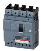
Circuit breaker 3VA6 UL Frame 600 breaking capacity class H 65kA @ 480V 4-pole, Line protection ETU830, LIG, In=400A overload protection, 100% rated Ir=160A...400A Short-circuit protection li=1.5...12 x In Ground-fault protection lg=0.2...1 x In, tg=0.05-0.8s without connection
