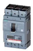
Circuit breaker 3VA6 UL Frame 600 breaking capacity class H 65kA @ 480 V 3-pole, Line protection ETU830, LIG, In=400A overload protection, 100% rated Ir=160A ...400A Short-circuit protection Ii=1.5...12 x In Ground-fault protection Ig=0.2... 1 x In, tg=0.05-0.8s cable connection on both sides
