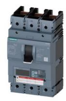
Circuit breaker 3VA6 UL Frame 600 breaking capacity class H 65kA @ 480V 3-pole, Line protection ETU830, LIG, In=400A overload protection, 100% rated Ir=160A...400A Short-circuit protection Ii=1.5...12 x In Ground-fault protection Ig=0.2...1 x In, tg=0.05-0.8s without connection
