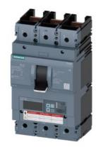
circuit breaker 3VA6 UL frame 600 breaking capacity class H 65kA @ 480V 3-pole, line protection ETU830, LIG, In=400A overload protection Ir=160A...400A short-circuit protection Ii=1.5...12 x In ground-fault protection Ig=0.2...1 x In, tg=0.05-0.8s without connection
