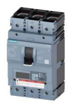
Circuit breaker 3VA6 UL Frame 600 breaking capacity class H 65kA @ 480 V 3pole, Line protection ETU556, LSI, In=400A overload protection, 100% rated Ir=160A ...400A Short-circuit protection Isd=0.6..10x In, Ii=1.5..12x In N conductor protection optionally with external CT; up to 160% Ground-fault alarm message via EFB300 or COM cable connection on both sides
