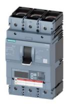
circuit breaker 3VA6 UL frame 600 breaking capacity class H 65kA @ 480 V 3-pole, line protection ETU556, LSI, In=400A overload protection Ir=160A ...400A short-circuit protection Isd=0.6..10x In, Ii=1.5..12x In N conductor protection opt. w. ext. CT; up to 160% ground-fault alarm message via EFB300 or COM cable connection on both sides
