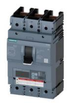
Circuit breaker 3VA6 UL Frame 600 breaking capacity class H 65kA @ 480V 3pole, Line protection ETU556, LSI, In=400A overload protection, 100% rated Ir=160A...400A Short-circuit protection Isd=0.6..10x In, Ii=1.5..12x In N conductor protection optionally with external CT, up to 160% Ground-fault alarm message via EFB300 or COM without connection
