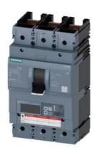
circuit breaker 3VA6 UL frame 600 breaking capacity class H 65kA @ 480V 3-pole, line protection ETU556, LSI, In=400A overload protection Ir=160A...400A short-circuit protection Isd=0.6..10x In, Ii=1.5..12x In N conductor protection optionally with external current transformer, up to 160% ground-fault alarm message via EFB300 or COM without connection
