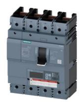
Circuit breaker 3VA6 UL Frame 600 breaking capacity class H 65kA @ 480V 4-pole, Line protection ETU560, LSIG, In=400A overload protection, 100% rated Ir=160A...400A Short-circuit protection Isd=0.6..10x In, Ii=1.5..12x In N conductor protection adjustable (OFF, up to 160%) Ground-fault protection Ig=0.2...1 x In= tg=0.05-0.8s without connection
