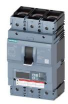
Circuit breaker 3VA6 UL Frame 600 breaking capacity class H 65kA @ 480 V 3pole, Line protection ETU560, LSIG, In=400A overload protection, 100% rated Ir=160A ...400A Short-circuit protection Isd=0.6..10x In, Ii=1.5..12x In N conductor protection optionally with external CT; up to 160% Ground-fault protection Ig=0.2... 1 x In, tg=0.05-0.8s cable connection on both sides
