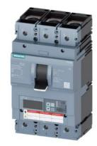
circuit breaker 3VA6 UL frame 600 breaking capacity class H 65kA @ 480 V 3pole, line protection ETU560, LSIG, In=400A overload protection Ir=160A ...400A short-circuit protection Isd=0.6..10x In, Ii=1.5..12x In N conductor protection opt. w. ext. CT; up to 160% ground-fault protection Ig=0.2... 1 x In, tg=0.05-0.8s cable connection on both sides
