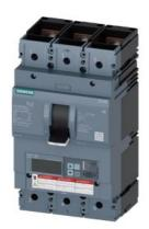
Circuit breaker 3VA6 UL Frame 600 breaking capacity class H 65kA @ 480 V 3-pole, Line protection ETU560, LSIG, In=400A overload protection, 100% rated Ir=160A ...400A Short-circuit protection Isd=0.6..10x In, Ii=1.5..12x In N conductor protection optionally with external CT; up to 160% Ground-fault protection Ig=0.2... 1 x In, tg=0.05-0.8s nut keeper kit on both sides
