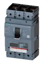
circuit breaker 3VA6 UL frame 600 breaking capacity class H 65kA @ 480 V 3pole, line protection ETU560, LSIG, In=400A overload protection Ir=160A ...400A short-circuit protection Isd=0.6..10x In, Ii=1.5..12x In N conductor protection opt. w. ext. CT; up to 160% ground-fault protection Ig=0.2... 1 x In, tg=0.05-0.8s nut keeper kit on both sides
