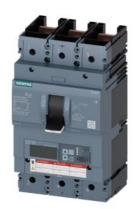
Circuit breaker 3VA6 UL Frame 600 breaking capacity class H 65kA @ 480V 3-pole, Line protection ETU560, LSIG, In=400A overload protection, 100% rated Ir=160A...400A Short-circuit protection Isd=0.6..10x In, Ii=1.5..12x In N conductor protection optionally with external CT, up to 160% Ground-fault protection Ig=0.2...1 x In, tg=0.05-0.8s without connection
