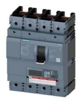
Circuit breaker 3VA6 UL Frame 600 breaking capacity class H 65kA @ 480V 4-pole, Line protection ETU550, LSI, In=400A overload protection, 100% rated Ir=160A...400A Short-circuit protection Isd=0.6..10x In, Ii=1.5..12x In N conductor protection adjustable (OFF, up to 150%) without connection
