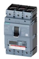
circuit breaker 3VA6 UL frame 600 breaking capacity class H 65kA @ 480 V 3-pole, line protection ETU550, LSI, In=400A overload protection Ir=160A ...400A short-circuit protection Isd=0.6..10x In, Ii=1.5..12x In N conductor protection opt. w. ext. CT; up to 160% cable connection on both sides
