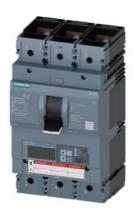
Circuit breaker 3VA6 UL Frame 600 breaking capacity class H 65kA @ 480 V 3-pole, Line protection ETU550, LSI, In=400A overload protection, 100% rated Ir=160A ...400A Short-circuit protection Isd=0.6..10x In, Ii=1.5..12x In N conductor protection optionally with external CT; up to 160% nut keeper kit on both sides
