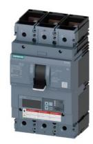
circuit breaker 3VA6 UL frame 600 breaking capacity class H 65kA @ 480 V 3-pole, line protection ETU550, LSI, In=400A overload protection Ir=160A ...400A short-circuit protection Isd=0.6..10x In, Ii=1.5..12x In N conductor protection opt. w. ext. CT; up to 160% nut keeper kit on both sides
