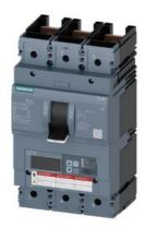
Circuit breaker 3VA6 UL Frame 600 breaking capacity class H 65kA @ 480V 3-pole, Line protection ETU550, LSI, In=400A overload protection, 100% rated Ir=160A...400A Short-circuit protection Isd=0.6..10x In, Ii=1.5..12x In N conductor protection optionally with external CT, up to 160% without connection
