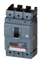
circuit breaker 3VA6 UL frame 600 breaking capacity class H 65kA @ 480V 3-pole, line protection ETU550, LSI, In=400A overload protection Ir=160A...400A short-circuit protection Isd=0.6..10x In, Ii=1.5..12x In N conductor protection optionally with external current transformer, up to 160% without connection
