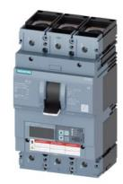
circuit breaker 3VA6 UL frame 400 breaking capacity class M 35kA @ 480 V 3pole, line protection ETU856, LSI, In=400A overload protection Ir=160A ...400A short-circuit protection Isd=0.6..10x In, Ii=1.5..10x In N conductor protection opt. w. ext. CT; up to 160% ground-fault alarm message via EFB300 or COM cable connection on both sides
