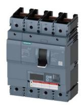
circuit breaker 3VA6 UL frame 400 breaking capacity class M 35kA @ 480V 4-pole, line protection ETU830, LIG, In=400A overload protection Ir=160A...400A short-circuit protection Ii=1.5...10 x In ground-fault protection Ig=0.2...1 x In, tg=0.05-0.8s without connection
