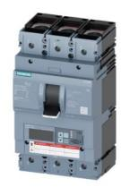
circuit breaker 3VA6 UL frame 400 breaking capacity class M 35kA @ 480 V 3-pole, line protection ETU830, LIG, In=400A overload protection Ir=160A ...400A short-circuit protection Ii=1.5...10 x In ground-fault protection Ig=0.2... 1 x In, tg=0.05-0.8s cable connection on both sides
