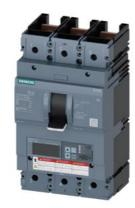
circuit breaker 3VA6 UL frame 400 breaking capacity class M 35kA @ 480V 3-pole, line protection ETU830, LIG, In=400A overload protection Ir=160A...400A short-circuit protection Ii=1.5...10 x In ground-fault protection Ig=0.2...1 x In, tg=0.05-0.8s without connection
