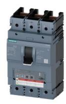
circuit breaker 3VA6 UL frame 400 breaking capacity class M 35kA @ 480V 3-pole, line protection ETU350, LSI, In=400A overload protection Ir=160A...400A short-circuit protection Isd=1.5...10 x Ir, Ii=10 x In without connection
