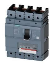
circuit breaker 3VA6 UL frame 400 breaking capacity class M 35kA @ 480V 4-pole, line protection ETU330, LIG, In=400A overload protection Ir=160A...400A short-circuit protection li=1.5...10 x In N conductor protection adjustable (OFF, 50%, 100%) ground-fault protection Ig=0.2...1 x In= tg=0.1/0.3s without connection
