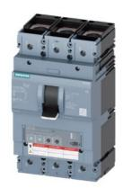
circuit breaker 3VA6 UL frame 400 breaking capacity class M 35kA @ 480 V 3-pole, line protection ETU330, LIG, ln=400A overload protection Ir=160A ...400A short-circuit protection Ii=1.5...10 x In ground-fault protection Ig=0.2... 1 x In, tg=0.1/0.3s cable connection on both sides
