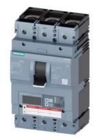
circuit breaker 3VA6 UL frame 400 breaking capacity class M 35kA @ 480 V 3pole, line protection ETU856, LSI, In=250A overload protection Ir=100A ...250A short-circuit protection Isd=0.6..10x In, Ii=1.5..12x In N conductor protection opt. w. ext. CT; up to 160% ground-fault alarm message via EFB300 or COM cable connection on both sides
