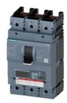
Circuit breaker 3VA6 UL frame 400 breaking capacity class M 35kA @ 480V 3pole, Line protection ETU856, LSI, In=250A overload protection, 100% rated Ir=100A...250A Short-circuit protection Isd=0.6..10x In, Ii=1.5..12x In N conductor protection optionally with external CT, up to 160% Ground-fault alarm message via EFB300 or COM without connection
