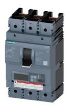
circuit breaker 3VA6 UL frame 400 breaking capacity class M 35kA @ 480V 3-pole, line protection ETU856, LSI, In=250A overload protection Ir=100A...250A short-circuit protection Isd=0.6..10x In, Ii=1.5..12x In N conductor protection optionally with external current transformer, up to 160% ground-fault alarm message via EFB300 or COM without connection
