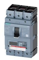
Circuit breaker 3VA6 UL frame 400 breaking capacity class M 35kA @ 480 V 3-pole, Line protection ETU850, LSI, In=250A overload protection, 100% rated Ir=100A ...250A Short-circuit protection Isd=0.6..10x In, Ii=1.5..12x In N conductor protection optionally with external CT; up to 160% cable connection on both sides
