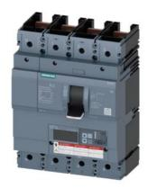
Circuit breaker 3VA6 UL frame 400 breaking capacity class M 35kA @ 480V 4-pole, Line protection ETU830, LIG, In=250A overload protection, 100% rated Ir=100A...250A Short-circuit protection Ii=1.5...12 x In Ground-fault protection Ig=0.2...1 x In, tg=0.05-0.8s without connection
