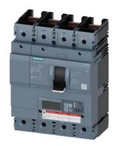
circuit breaker 3VA6 UL frame 400 breaking capacity class M 35kA @ 480V 4-pole, line protection ETU830, LIG, In=250A overload protection Ir=100A...250A short-circuit protection Ii=1.5...12 x In ground-fault protection Ig=0.2...1 x In, tg=0.05-0.8s without connection
