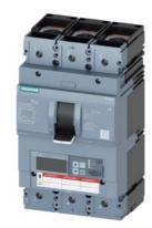
Circuit breaker 3VA6 UL frame 400 breaking capacity class M 35kA @ 480 V 3-pole, Line protection ETU830, LIG, In=250A overload protection, 100% rated Ir=100A ...250A Short-circuit protection Ii=1.5...12 x In Ground-fault protection Ig=0.2... 1 x In, tg=0.05-0.8s cable connection on both sides
