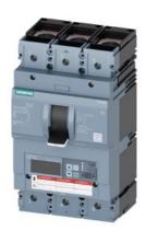
circuit breaker 3VA6 UL frame 400 breaking capacity class M 35kA @ 480 V 3-pole, line protection ETU830, LIG, ln=250A overload protection Ir=100A ...250A short-circuit protection li=1.5...12 x ln ground-fault protection lg=0.2... 1 x ln, tg=0.05-0.8s cable connection on both sides
