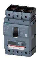
circuit breaker 3VA6 UL frame 400 breaking capacity class M 35kA @ 480 V 3-pole, line protection ETU830, LIG, In=250A overload protection Ir=100A ...250A short-circuit protection Ii=1.5...12 x In ground-fault protection Ig=0.2... 1 x In, tg=0.05-0.8s nut keeper kit on both sides
