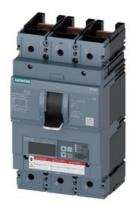
Circuit breaker 3VA6 UL frame 400 breaking capacity class M 35kA @ 480V 3-pole, Line protection ETU830, LIG, In=250A overload protection, 100% rated Ir=100A...250A Short-circuit protection Ii=1.5...12 x In Ground-fault protection Ig=0.2...1 x In, tg=0.05-0.8s without connection
