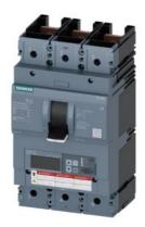
circuit breaker 3VA6 UL frame 400 breaking capacity class M 35kA @ 480V 3-pole, line protection ETU830, LIG, In=250A overload protection Ir=100A...250A short-circuit protection Ii=1.5...12 x In ground-fault protection Ig=0.2...1 x In, tg=0.05-0.8s without connection
