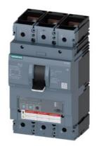
Circuit breaker 3VA6 UL frame 400 breaking capacity class M 35kA @ 480 V 3-pole, Line protection ETU320, LI, In=250A overload protection, 100% rated Ir=100A ...250A Short-circuit protection Ii=1.5...12 x In nut keeper kit on both sides
