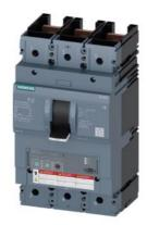
Circuit breaker 3VA6 UL frame 400 breaking capacity class M 35kA @ 480V 3-pole, Line protection ETU320, LI, In=250A overload protection, 100% rated Ir=100A...250A Short-circuit protection Ii=1.5...12 x In without connection
