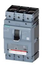
circuit breaker 3VA6 UL frame 400 3-pole, starter protection ETU310M, I, In=250A without overload protection short-circuit protection li=3...15 x In cable connection on both sides
