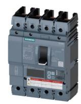
Circuit breaker 3VA6 UL frame 250 breaking capacity class C 100kA @ 480V 4pole, Line protection ETU856, LSI, In=250A overload protection, 100% rated Ir=100A...250A Short-circuit protection Isd=0.6..10x In, Ii=1.5..10x In N conductor protection adjustable (OFF, up to 100%) Ground-fault alarm message via EFB300 or COM without connection
