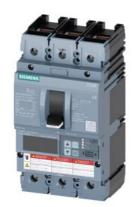
Circuit breaker 3VA6 UL frame 250 breaking capacity class C 100kA @ 480 V 3pole, Line protection ETU856, LSI, In=250A overload protection, 100% rated Ir=100A ...250A Short-circuit protection Isd=0.6..10x In, Ii=1.5..10x In N conductor protection optionally with external CT; up to 160% Ground-fault alarm message via EFB300 or COM cable connection on both sides
