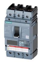
circuit breaker 3VA6 UL frame 250 breaking capacity class C 100kA @ 480 V 3pole, line protection ETU856, LSI, In=250A overload protection Ir=100A ...250A short-circuit protection Isd=0.6..10x In, Ii=1.5..10x In N conductor protection opt. w. ext. CT; up to 160% ground-fault alarm message via EFB300 or COM cable connection on both sides
