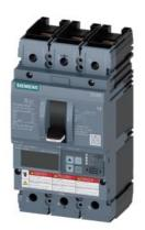
Circuit breaker 3VA6 UL frame 250 breaking capacity class C 100kA @ 480 V 3-pole, Line protection ETU856, LSI, In=250A overload protection, 100% rated Ir=100A ...250A Short-circuit protection Isd=0.6..10x In, Ii=1.5..10x In N conductor protection optionally with external CT; up to 160% Ground-fault alarm message via EFB300 or COM nut keeper kit on both sides
