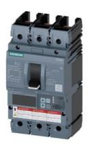
Circuit breaker 3VA6 UL frame 250 breaking capacity class C 100kA @ 480V 3-pole, Line protection ETU856, LSI, In=250A overload protection, 100% rated Ir=100A...250A Short-circuit protection Isd=0.6..10x In, Ii=1.5..10x In N conductor protection optionally with external CT, up to 160% Ground-fault alarm message via EFB300 or COM without connection
