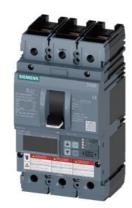
Circuit breaker 3VA6 UL frame 250 breaking capacity class C 100kA @ 480 V 3pole, Line protection ETU860, LSIG, In=250A overload protection, 100% rated Ir=100A ...250A Short-circuit protection Isd=0.6..10x In, Ii=1.5..10x In N conductor protection optionally with external CT; up to 160% Ground-fault protection Ig=0.2... 1 x In, tg=0.05-0.8s nut keeper kit on both sides
