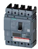
Circuit breaker 3VA6 UL frame 250 breaking capacity class C 100kA @ 480V 4-pole, Line protection ETU850, LSI, In=250A overload protection, 100% rated Ir=100A...250A Short-circuit protection Isd=0.6..10x In, Ii=1.5..10x In N conductor protection adjustable (OFF, up to 100%) without connection
