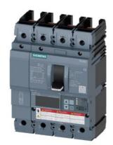
Circuit breaker 3VA6 UL frame 250 breaking capacity class C 100kA @ 480V 4-pole, Line protection ETU830, LIG, In=250A overload protection, 100% rated Ir=100A...250A Short-circuit protection li=1.5...10 x In Ground-fault protection lg=0.2...1 x In, tg=0.05-0.8s without connection
