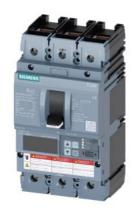
Circuit breaker 3VA6 UL frame 250 breaking capacity class C 100kA @ 480 V 3pole, Line protection ETU830, LIG, In=250A overload protection, 100% rated Ir=100A ...250A Short-circuit protection Ii=1.5...10 x In Ground-fault protection Ig=0.2... 1 x In, tg=0.05-0.8s cable connection on both sides
